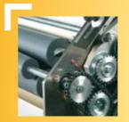
The drivers and adjusting devices for the belts and rolling cylinders are of a particularly robust construction, and supported by aluminium sidewalls milled from the block. The feeding cylinder which is shaped like a spindle and the nondeforming belt ensure both accuracy and conformity in the finished products.
